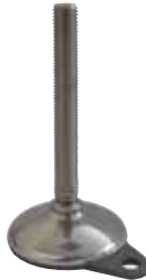
Part. R0748F - Pag. R37 Ø 100 • Stainless steel • Hygiene • Prefitting for fixing • Max. load 25000 N.
