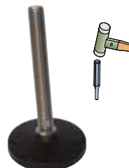
Part. R0134 - Pag. R20 Ø 100 • Prefitting for fixing • Max. load 20000 N.
